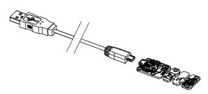
You must plug in your Colswe-Temperaturemodule with a USB-A to USB micro B cable
